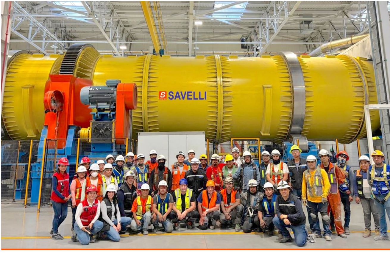
Savelli Technologies S.r.l. - Rotary cooling drum to cool sand and castings for a new foundry in Mexico
