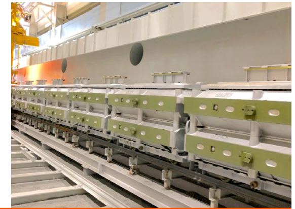
Savelli Technologies S.r.l. - Horizontal flask moulding line for the production of truck engine blocks and cylinder heads in Sweden
