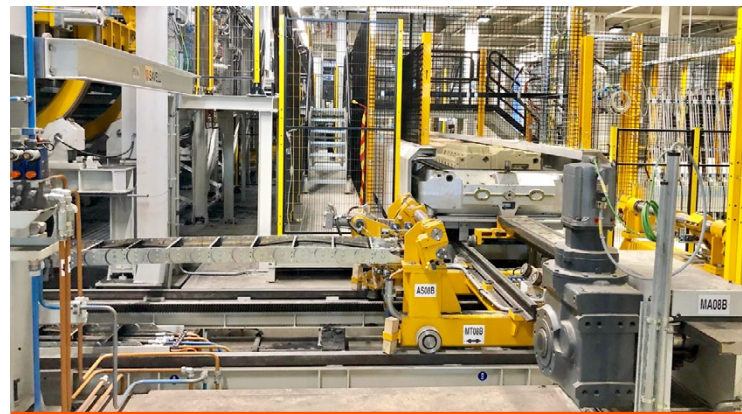
Savelli Technologies S.r.l. - Horizontal flask moulding line for the production of truck engine blocks and cylinder heads in Sweden
